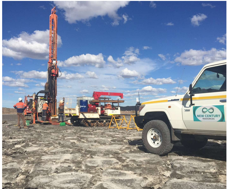
Figure 4: Tailings drilling at the Century Zinc Mine
