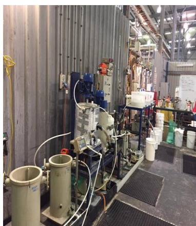
Phosphoric Acid Regeneration Circuit
