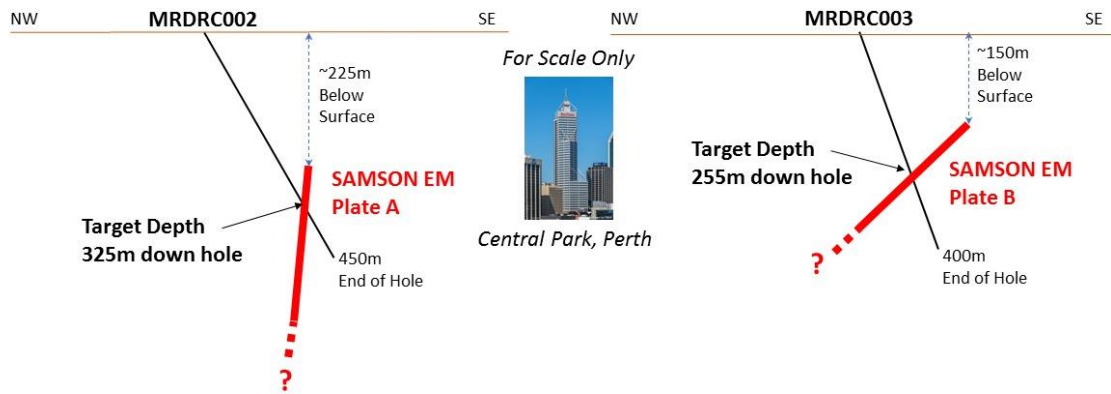
Figure 4. Section view of planned RC drill holes, MRDRC002 and 003, to target HP-MLTEM SAMSON conductive plate models A and B, Tyrrell's target area. Modelled conductive plates A and B on Lines 8B and 9B were interpreted to represent high conductance (4-6000 Siemens) bedrock features with at least 150m modelled depth extent down plunge.
