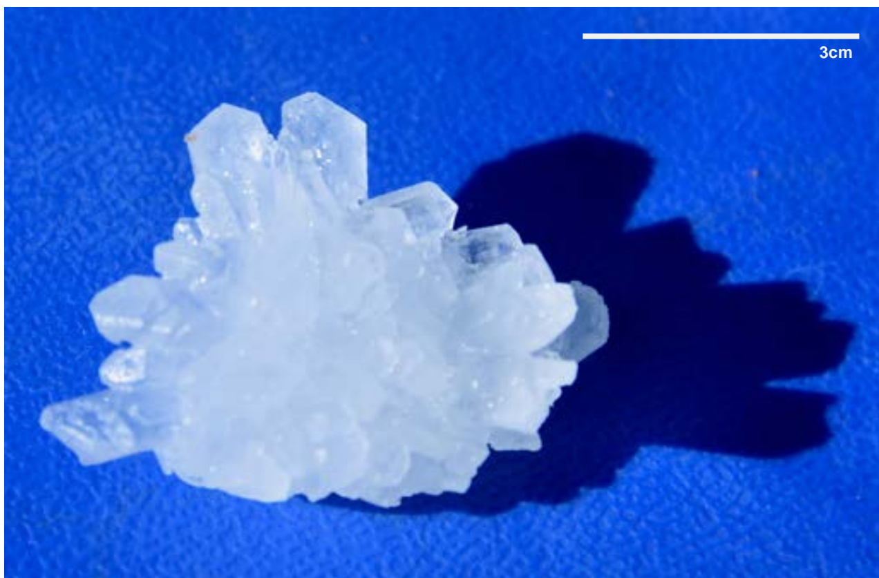
Figure 5: Sample of Salt Crystal Containing Kainite from Lake Wells Site Evaporation Trial
