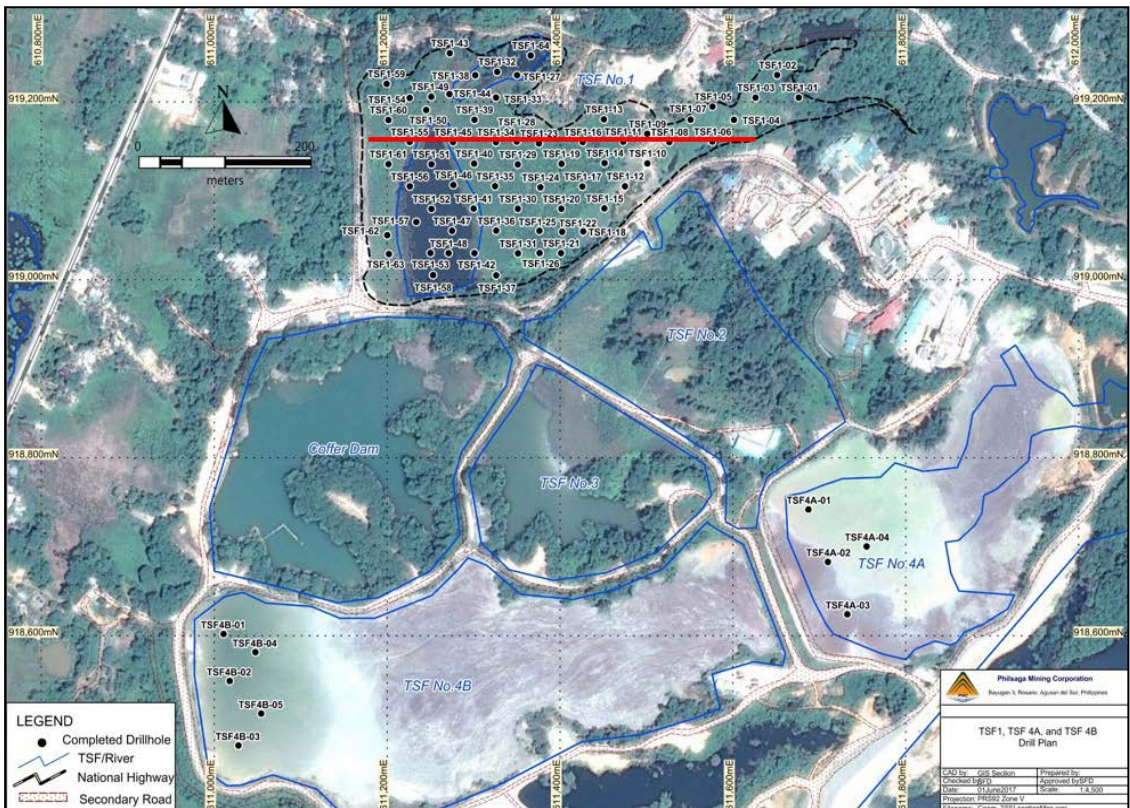
Figure 8. Location of completed drill holes in TSF 1, TSF 4A and TSF 4B.
