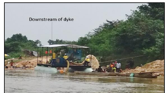
Figure 2. Gbinima dredging Project, EL 15/2012 (above, at left and inset). The planned dredge sites (red diamonds at left) have been preferentially selected on the basis of the Sewa River bedrock topography (e.g. dolerite dyke, at left) and suspected gravel fill from historic bathymetric and ground penetrating radar (GPR) survey results. The site of the current dredging activities at the ‘Cookie Jar’ alluvial flat is shown in dashed red line. (cf. Fig. 2).
