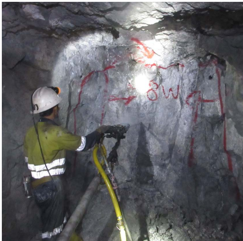
Figure 5. Airleg miner operating in hanging wall drive on Level 8.
