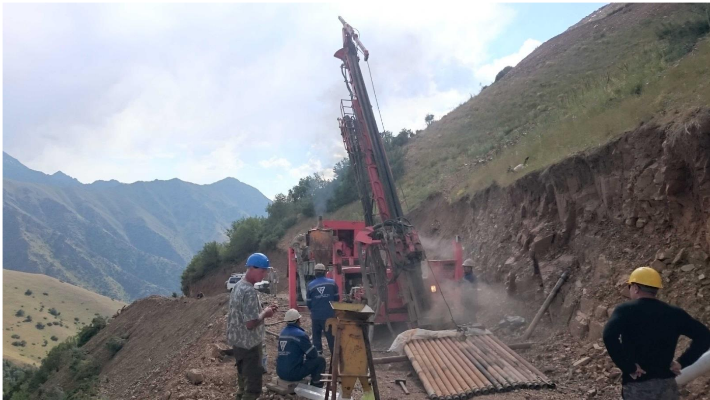
Figure 2: Drill rig completing ERC17-001 at the Quartz Zone. The copper oxide malachite was identified from 12-26 metres and native copper was identified at 34 metres.
