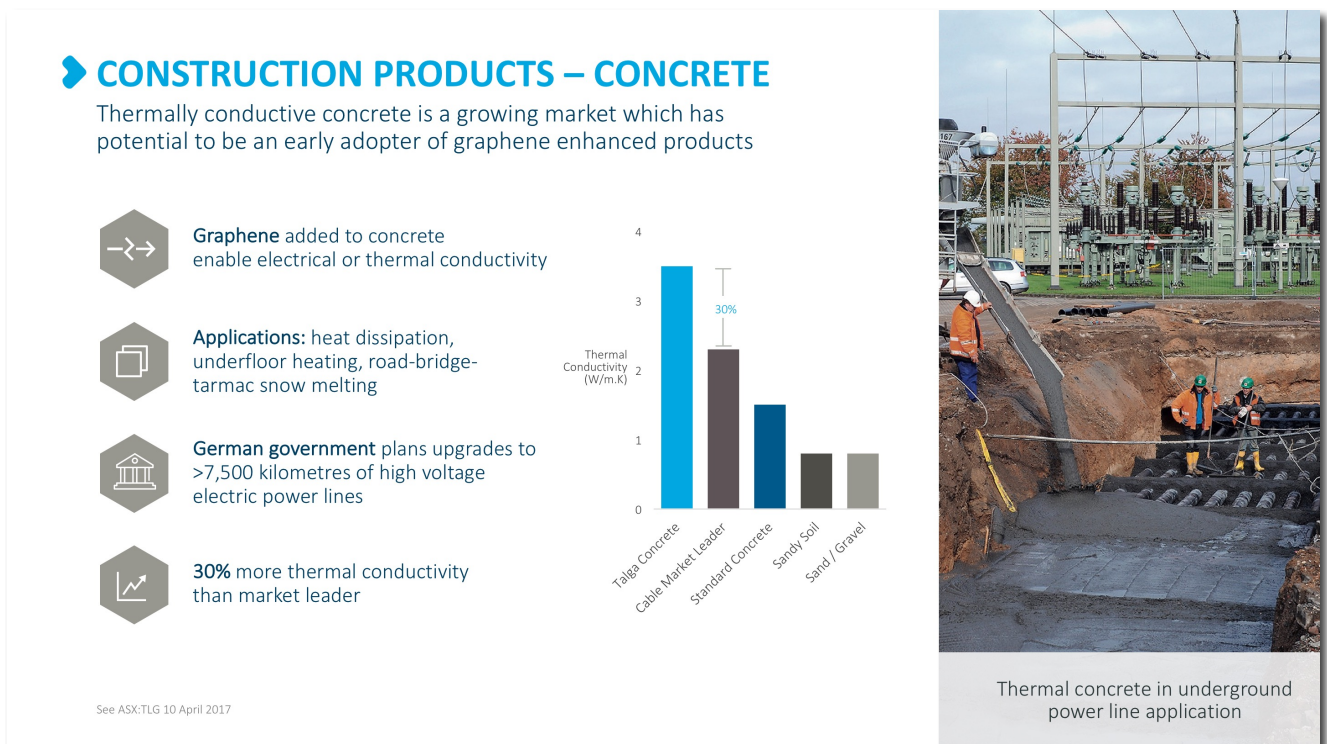
Figure 2. Talga graphene and graphite products increase thermal conductivity of concrete to enable power cables to be buried underground and improve heat dispersion, power efficiency and costs.
