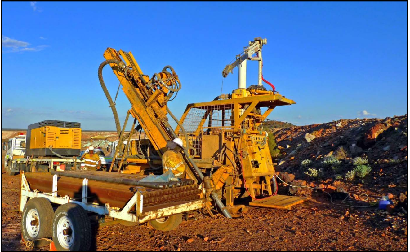
Figure 3. Specialty RC drill rig capable of drilling low-angle holes.
