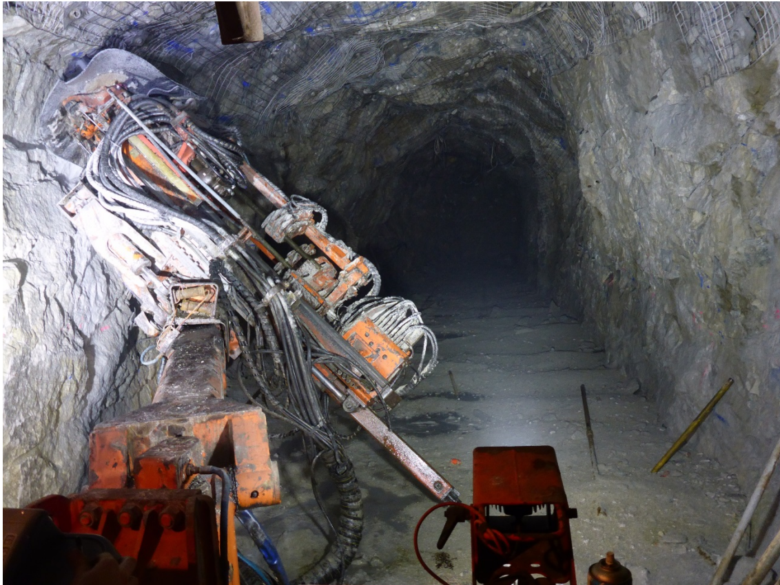
Figure 1. Solo Drilling Rig in the Long Hole Stope at the A1 Gold Mine
