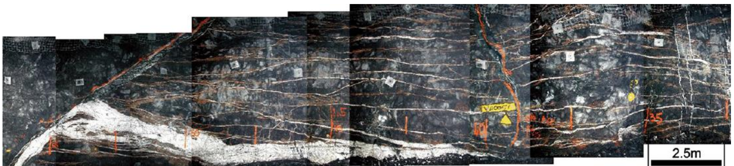
Figure 10: Darlot Centenary orebody 1100 level underground face photo mosaic showing sub-horizontal moderately dipping veins (Kenworthy, Hagemann 2007)
