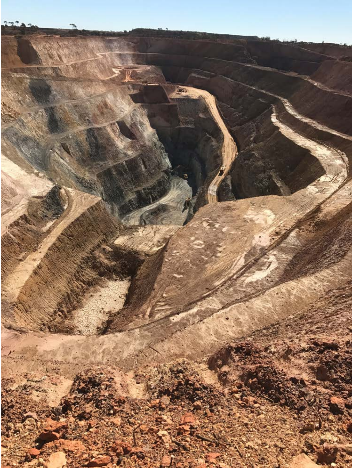
Figure 3 - Monday July 31, 2017 showing work on the 325mRL (designed pit floor 315mRL and surface 440mRL) of the Zoroastrian Central Pit Looking North.
