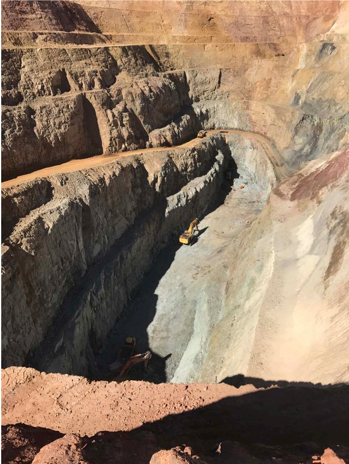
Figure 4- Monday July 31, 2017 showing work on the 325mRL (designed pit floor 315mRL and surface 440mRL) of the Zoroastrian Central Pit Looking South.
