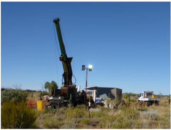
Figure 1: Photo of diamond drill rig at the Grapple Prospect
