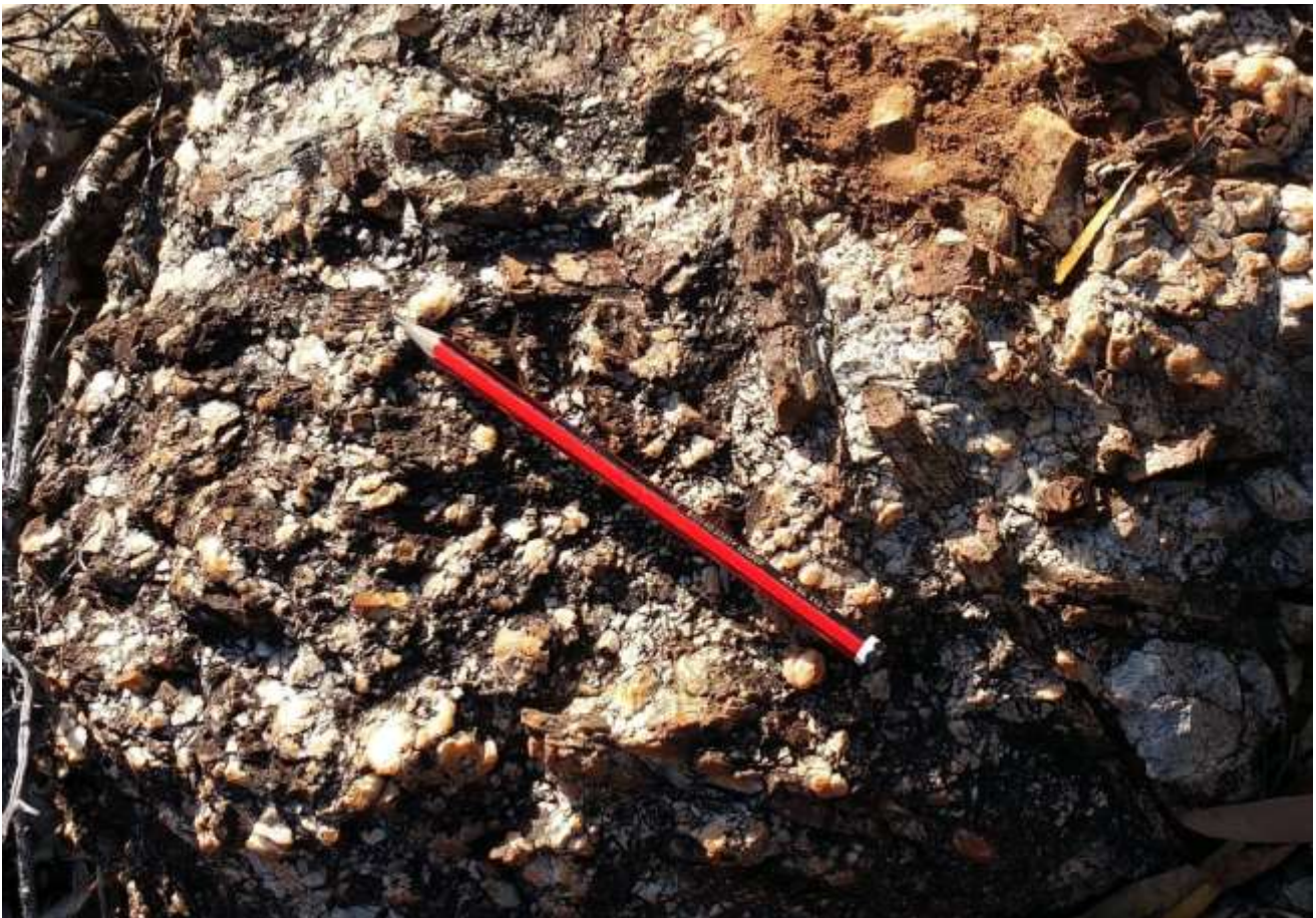
Figure 1. Photo of outcropping spodumene bearing pegmatite at Bravo Cluster near sample site AP00406. The darker coloured rod shaped crystals below and right of the pencil, and the dark blotches left of the pencil, are spodumene.
