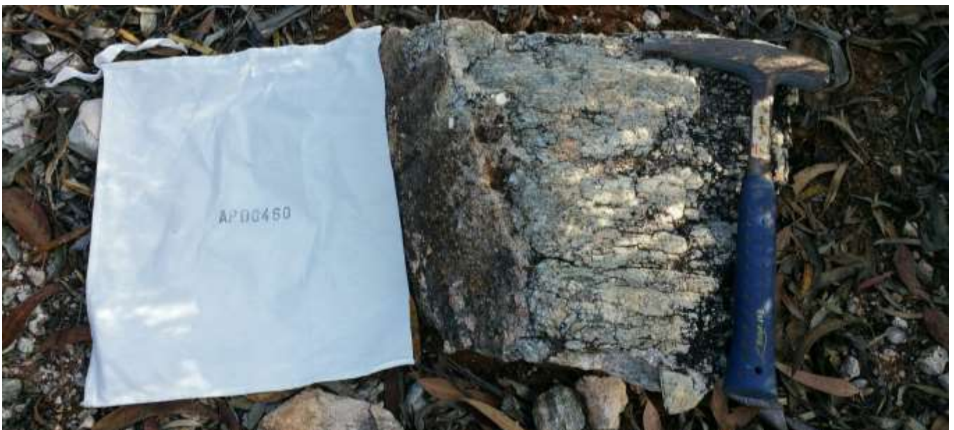
Figure 3. Photo of the AP00460 sample site, which returned 1.89% \text{Li}_2\text{O} . The greenish hewed material on the right hand 80% of this sample contains abundant spodumene. This specimen was taken from an historic costean.
