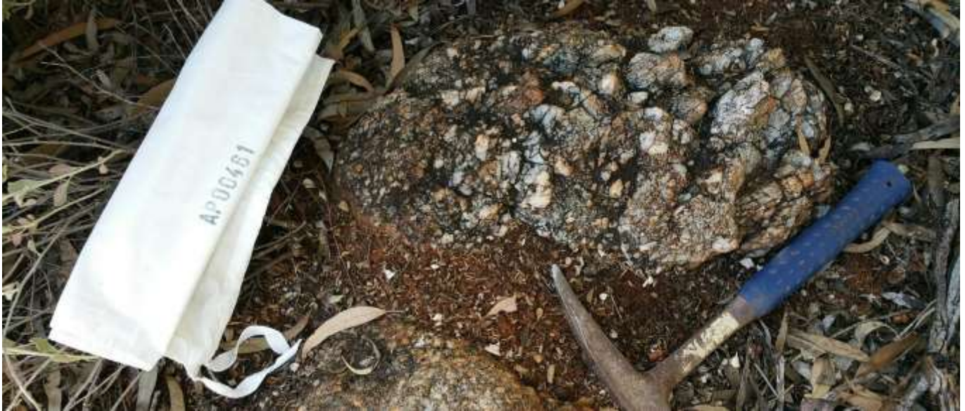
Figure 2. Photo of the AP00461 sample site, which returned 3.40% \text{Li}_2\text{O} . The orange brown tarnished crystals above the hammer are spodumene
