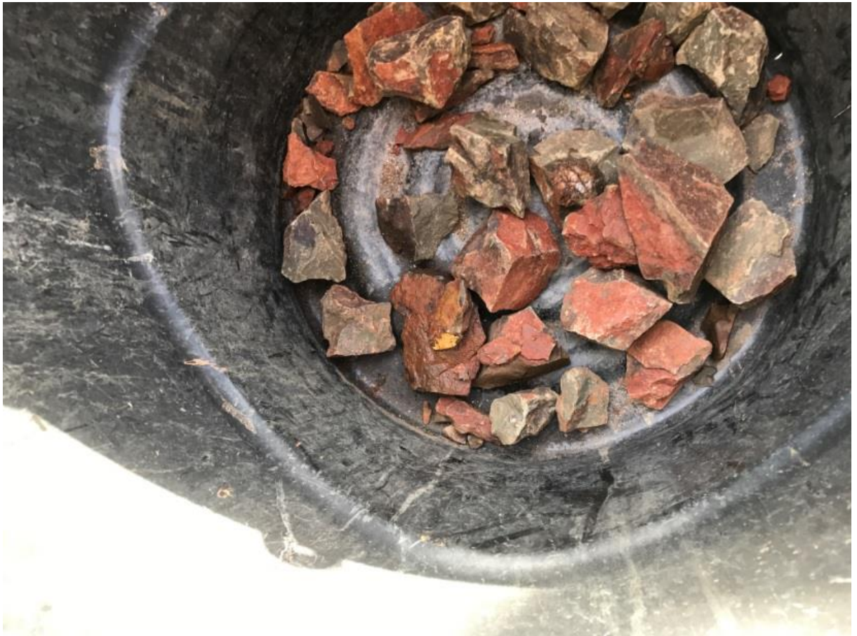
(Figure 3: Sorted Concentrate immediately following separation.)
