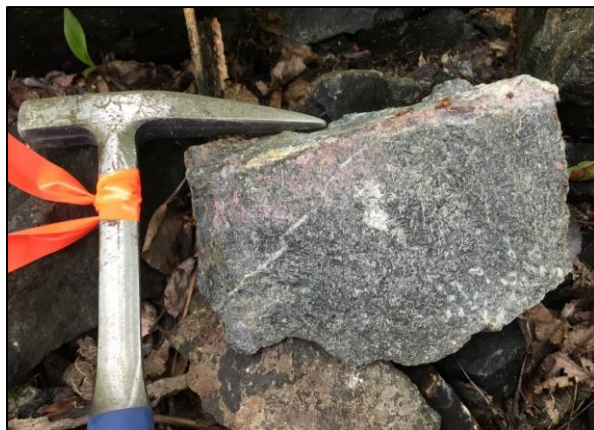
Image 7: Cobalt bloom on rock sample taken at the Van Chester (Last Chance) Prospect
