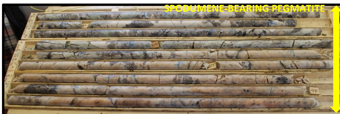
Figure 1. Drill core obtained from drill hole SL-17-22 (37.3m to 49.3m) showing the intersection of high-quality spodumene-bearing pegmatite, (including the intercept grading 5.7% \text{Li}_2\text{O} at 41.90m down hole).
