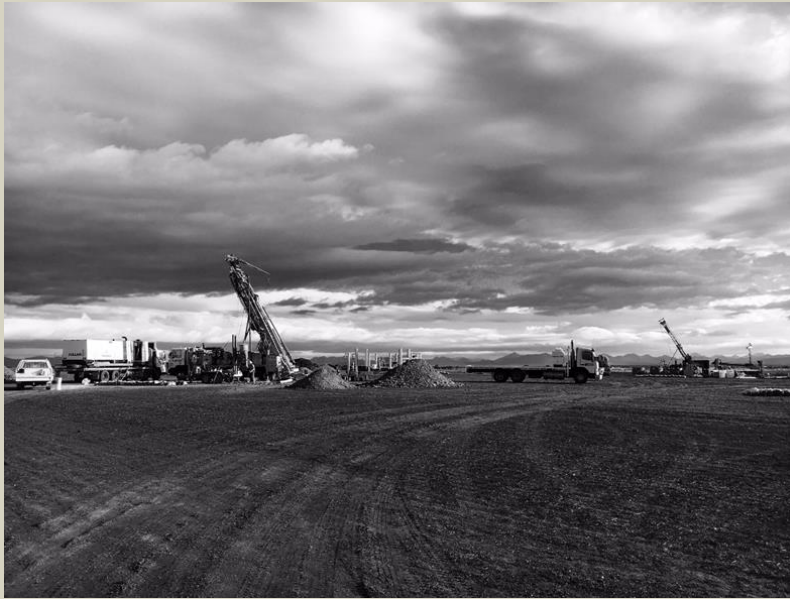
Photo 1. RC Drill rig (foreground) and diamond rig (background) at the Thursday's Gossan prospect, May 2017.
