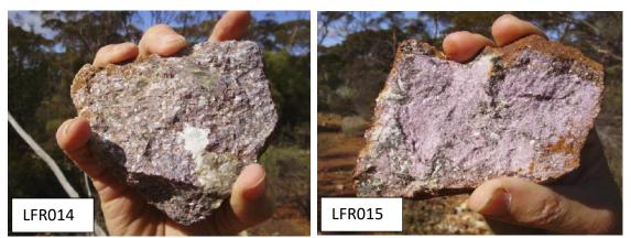
**Figures 2 and 3**. Li-mica (lepidolite) in pegmatite from the Lefroy prospect. Samples grade 3.14% Li2O (LFR014) and 3.55% Li2O (LFR015). From MXR ASX announcement dated 23 May 2016.
