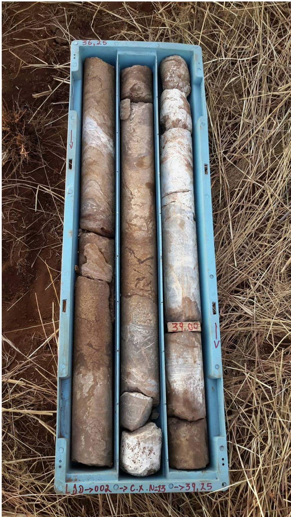
Hole LJD002 – CORE 36.25m- 39.25m grading 15.08% TREO
