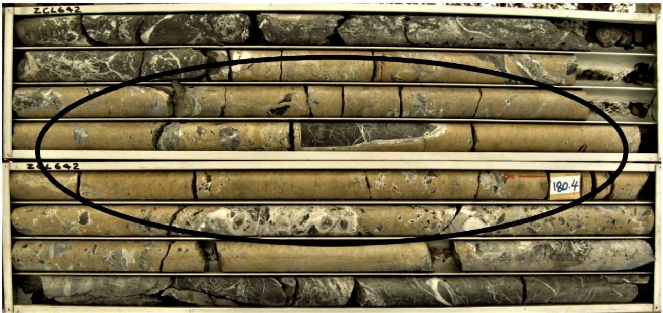
Figure 4: Hole ZCL642 showing massive sphalerite mineralisation (honey colour) within the interval 174-183m grading 27.5% Zn + Pb
