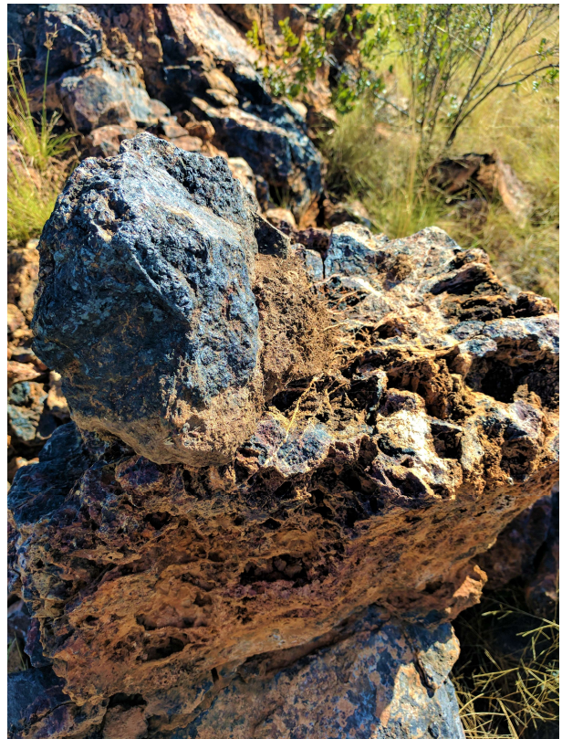
Figure 5: Perspective of the Watsons Lode veins, looking to the south-west, and close-up of the lode near Watsons shaft, showing the quartz vein with abundant cavities after sphalerite and carbonate.
