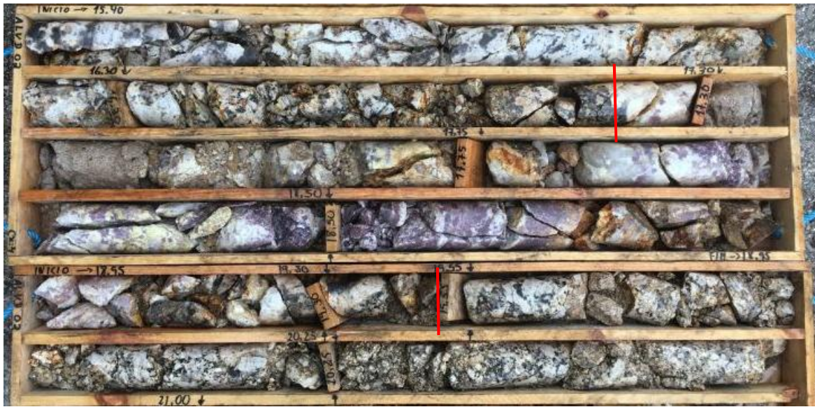
Figure 2. Lepidolite-bearing pegmatite (ALVD02, Block 1, Sill M), 2.35 m @ 1.41% \text{Li}_2\text{O} from 17.20 m; 15% lepidolite (estimated).
