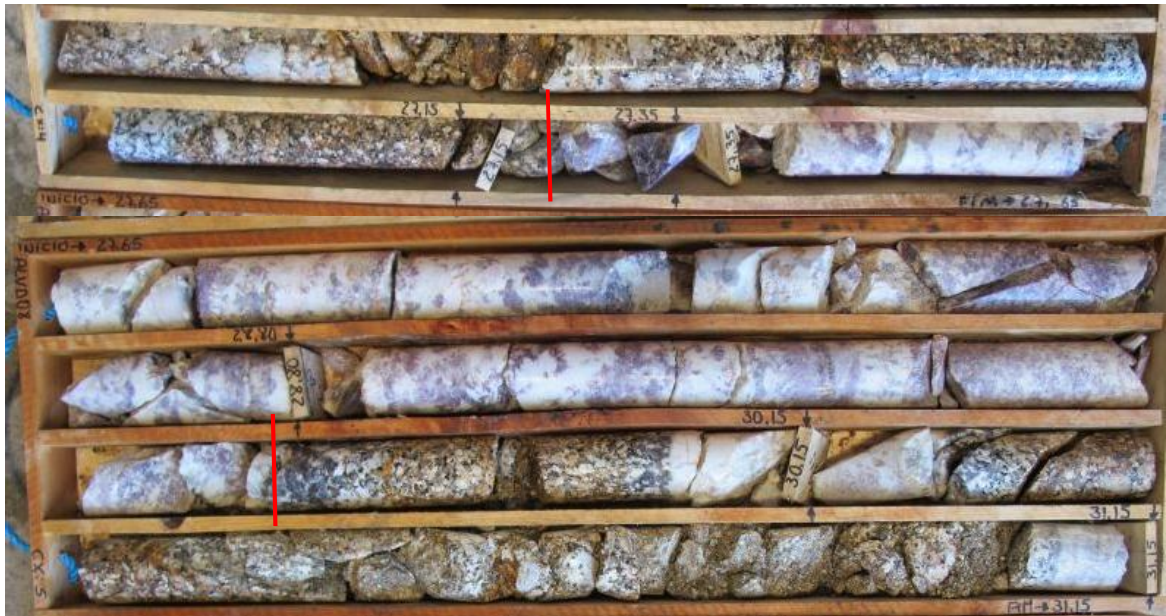
Figure 3. Lepidolite-bearing pegmatite (ALVD08, Block 1, Sill L), 2.55 m @ 1.30 \text{Li}_2\text{O} from 27.2 m; 15% lepidolite (estimated).
