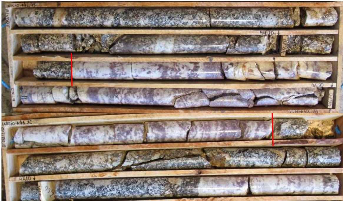
Figure 4. Lepidolite-bearing pegmatite (ALVD08, Block 1, Sill M), 2.55 m @ 1.76% \text{Li}_2\text{O} from 44.45 m; 30% lepidolite (estimated).
