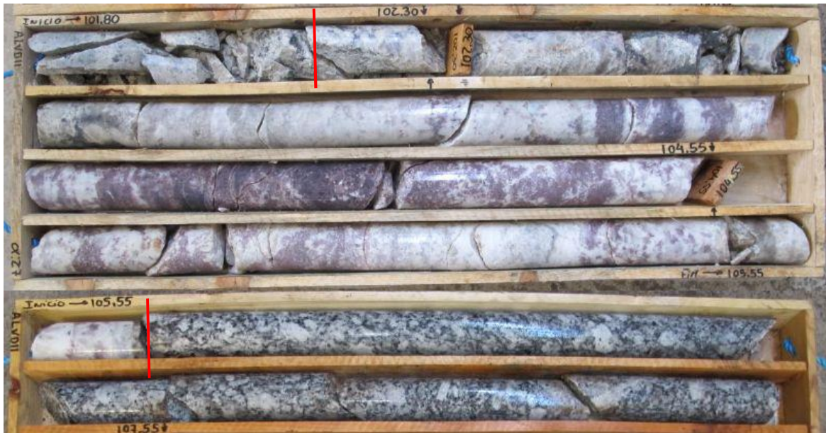
Figure 5. Lepidolite-bearing pegmatite (ALVD11, Block 3, identified as Sill N), 3.58 m @ 1.07% \text{Li}_2\text{O} from 102.13 m; 15% lepidolite (estimated).
