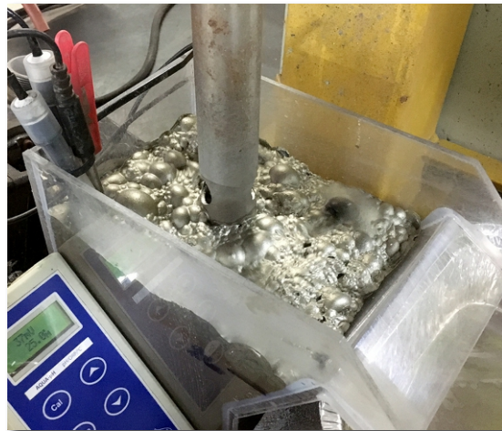
Figure 1 Flotation testing of cobalt-bearing sulphides from Kiskama project.
