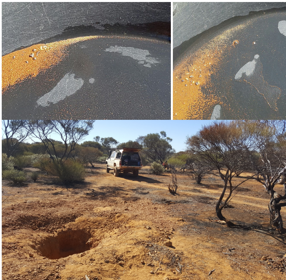
Figure 1 Photos of large gold tail from crushed laterite and pit in laterite,
