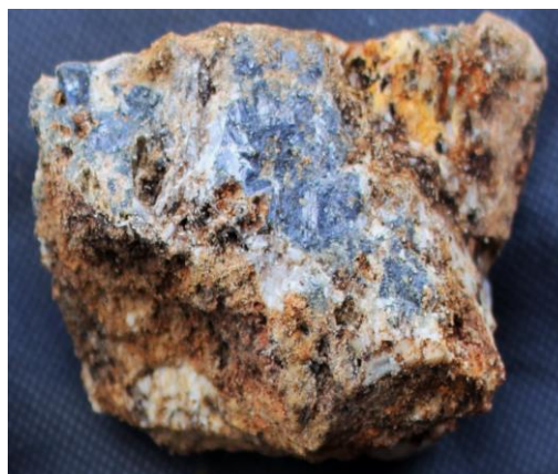
Figure 3: RIGHT Hand specimen of the NS vein exposed in the underground mine working showing coarse sulphides and gossan after sulphides. FAR RIGHT The NS vein, that is exposed in the underground working, occurring at surface.
