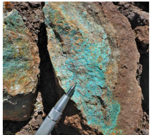
Figure 5: RIGHT Hand specimen of a volcanic rock showing strong secondary copper mineralisation.
