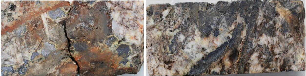
Figure 1: Core photos of different forms of mineralisation in RDDH-013. ABOVE LEFT Coarse galena (grey) with smithsonite rims (pale green). ABOVE RIGHT Fine-grained galena (grey) occurring with barite-calcite gangue material.
