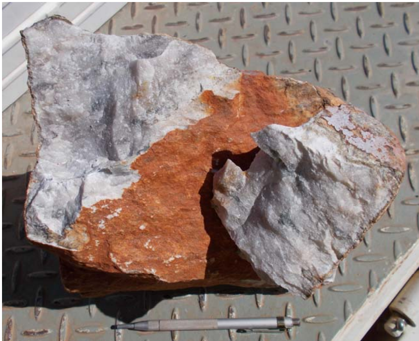
Figure 3: Rock chip previously collected from section A-A' grading 3.77% Li 2 O (see Figure 4)
