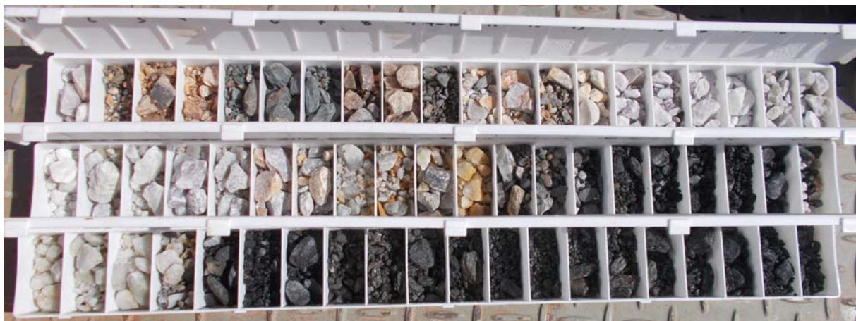
Figure 5: GASRC0004 Showing the top 60m including pegmatites from 0m-4m, 7m-31m and 39m-44m
