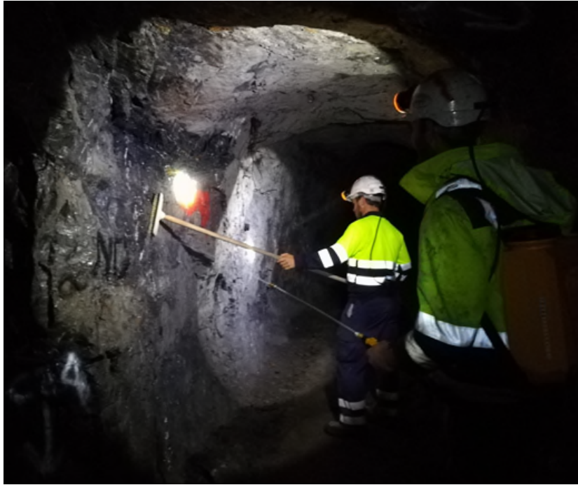
Figure 1: Cleaning the face of historical access revealing the underlying mineralisation to be sampled.
