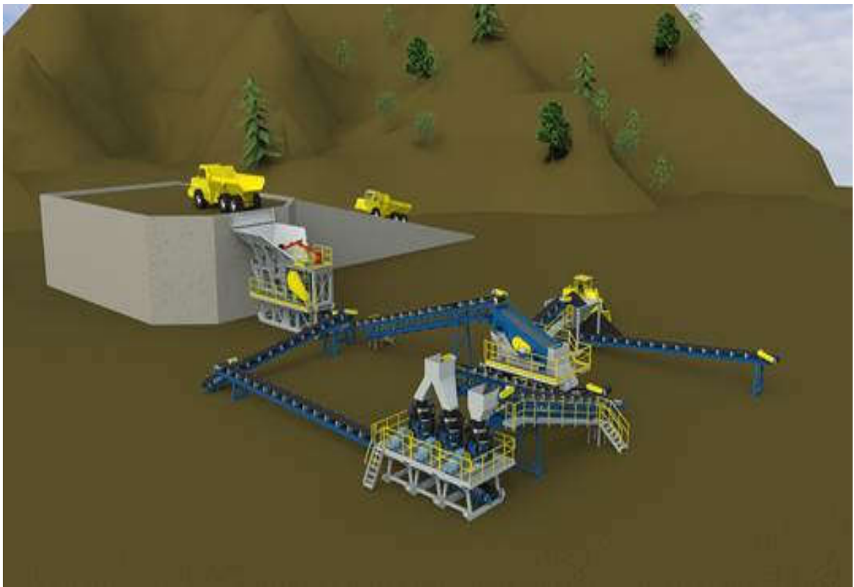
Diagram 7: Sepro Systems 75 tph three stage crushing circuit.
