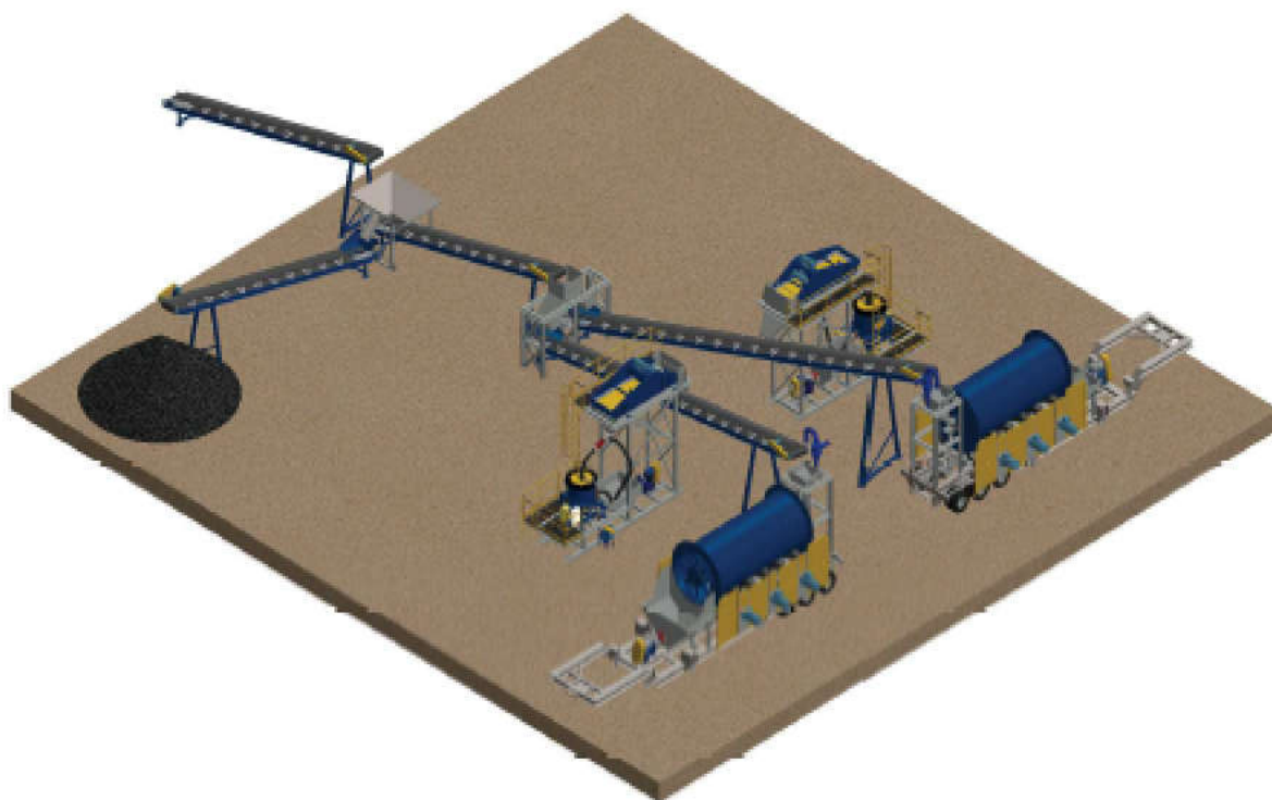
Diagram 8: Sepro Systems 40 tph grinding and gravity plant (dual stream mills and centrifugal concentrators).
