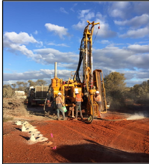
Figure 3: Combination aircore/RC drill rig at T1 gold prospect
