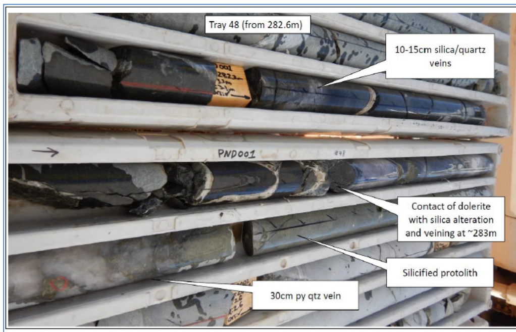
Figure 4. Tray 48 PND001 Photo showing the nature of the breccia contact and veining including texturally destructive silicification
