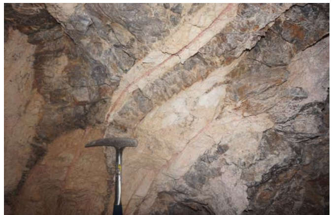
Figure 4 and 5. Weathered spodumene in underground workings at Geminis mine
