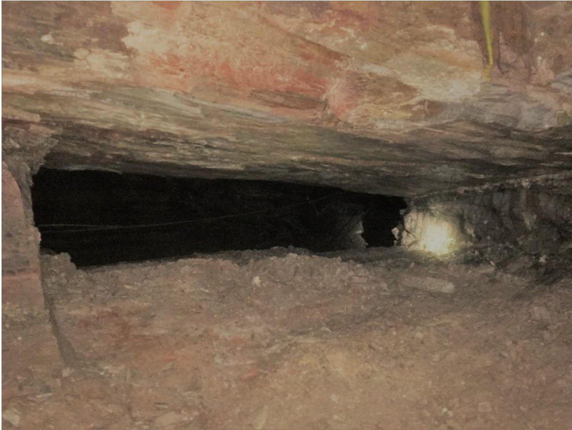
Figure 1: L3N stope trial – stope width of 0.5m achieved
