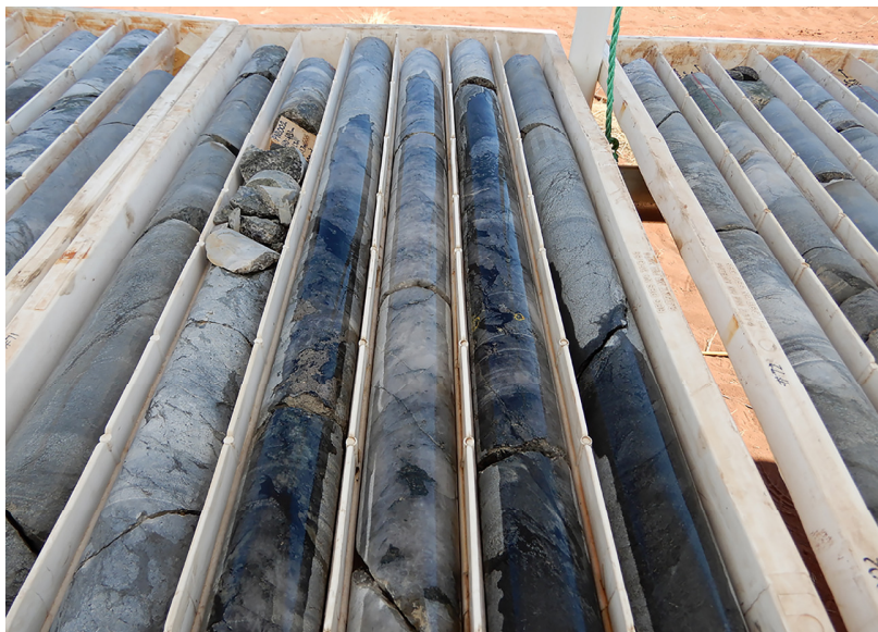
Figure 1: Core from PND002 showing strong quartz-biotite-chlorite-pyrrhotite-chalcopyrite veining and alteration
