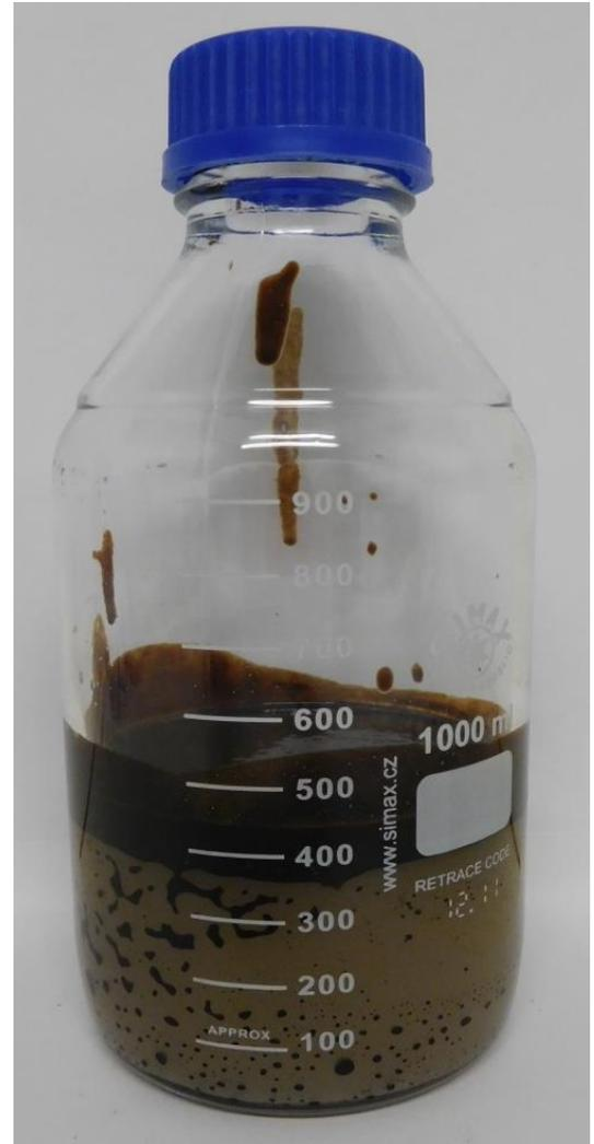
Xanadu-1 oil and oil-cut mud recovered from 1576.9 mMDRT in the Irwin River Coal Measures “A” sand with the Schlumberger Saturn Probe wireline tool. Further oil samples from this zone have been sent for analysis in Perth.
