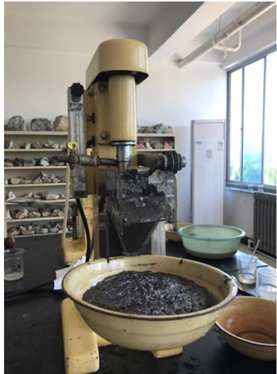
Figure 1: Flotation Optimisation Testwork currently in progress at Xinhai Laboratory, Yantai, China
