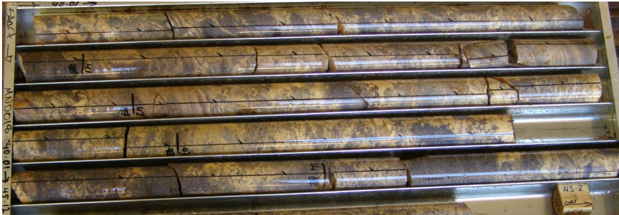
Figure 12 – Diamond core from MND018 showing zone of purple coloured lepidolite. Sampling of this zone returned the highest assay result of 2.14% Li 2 O from 43.36m to 44m. Photo shows diamond core from 40.01m to 45.12m.
