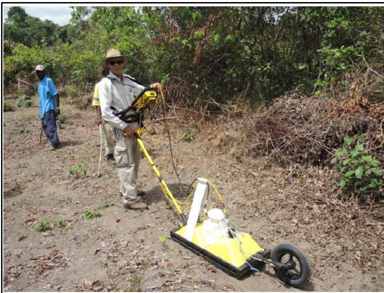
Figure 13. GPR survey in progress (deployment of 250 MHz GPR Antenna, at left; 100 MHz Antenna at right).
