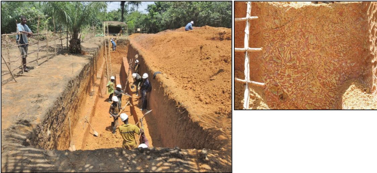
Figure 33. Excavation of trench (at left), over probe-positive KIM soil-sampling results for the POD011 AM geophysical anomaly, EL 11/2014. The causative magnetic body proved to be a diabase dyke (Elephant-skin alteration, at right). The source of the KIM ilmenites in the overlying soil horizon, is yet to be resolved.
