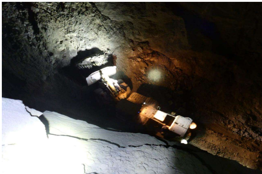
Figure 5. View from 1394 Level of the Tele Remote Control Bagger loading Ore in the Long Hole Stope on the 1380 Level at the A1 Mine
