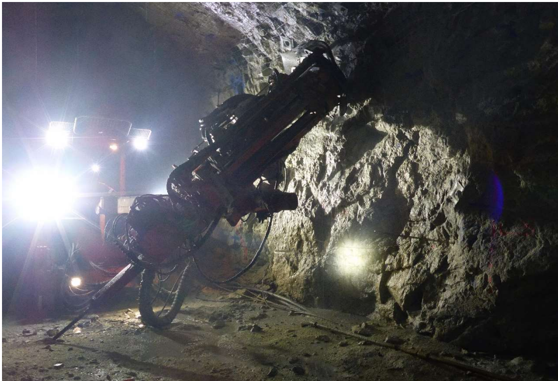
Figure 3. Long Hole Rig drilling the 1394 Long Hole Stope between 1394 to 1410 Levels.
