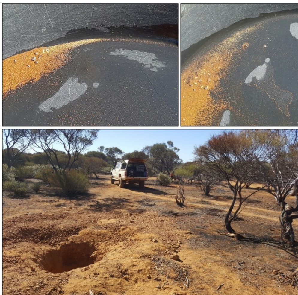
Figure 2 Photos of large gold tail from crushed laterite in pit at Mertondale.
