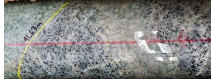
Potassic alteration comprising K-Feldspar (pale pink) and secondary Biotite (black) overprinting earlier diorite ZM17010 91.6m
