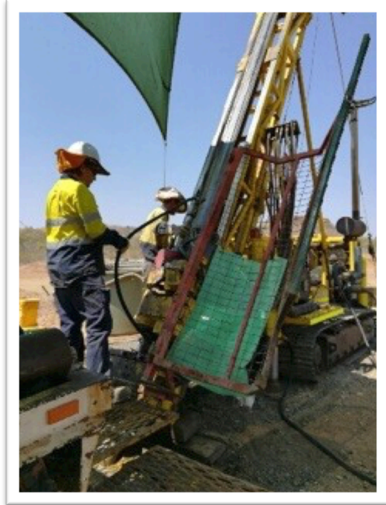
Diamond Core Drilling at Mt Freda
