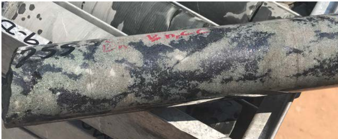
Figure 4: Drill core from MO-G-80D at current western limit of T3 drilling showing strong chalcocite/bornite mineralisation within sandstone host at approximately 255m down hole depth.
