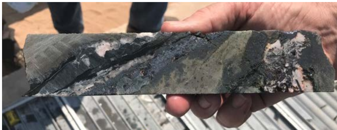
Figure 5: Drill core from hole MO-G-76D at eastern limit of T3 drilling showing strong chalcocite vein mineralisation within mudstone at approximately 346.6m down hole depth.
