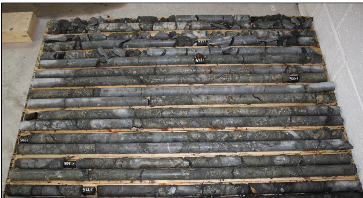
Figure 2: Massive sulphides in Z_4069_008 at the McGregor Prospect. From 497.0m to 500.7m down-hole (visual estimate, sphalerite, tan, 9%, galena 1-2%, marcasite, greenish, 25%); 502.40 to 509.05 (visual estimates, sphalerite, 9%, galena 2-4%, marcasite, 15-18%) and 509.05 to 511.90 (visual estimates, sphalerite, 4%, galena 2%, marcasite, 50%).
