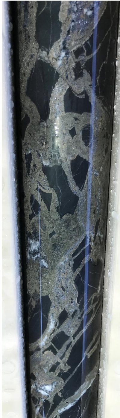
Figure Five – Fault Controlled Zinc and Lead Mineralisation in Hole BB04-17
