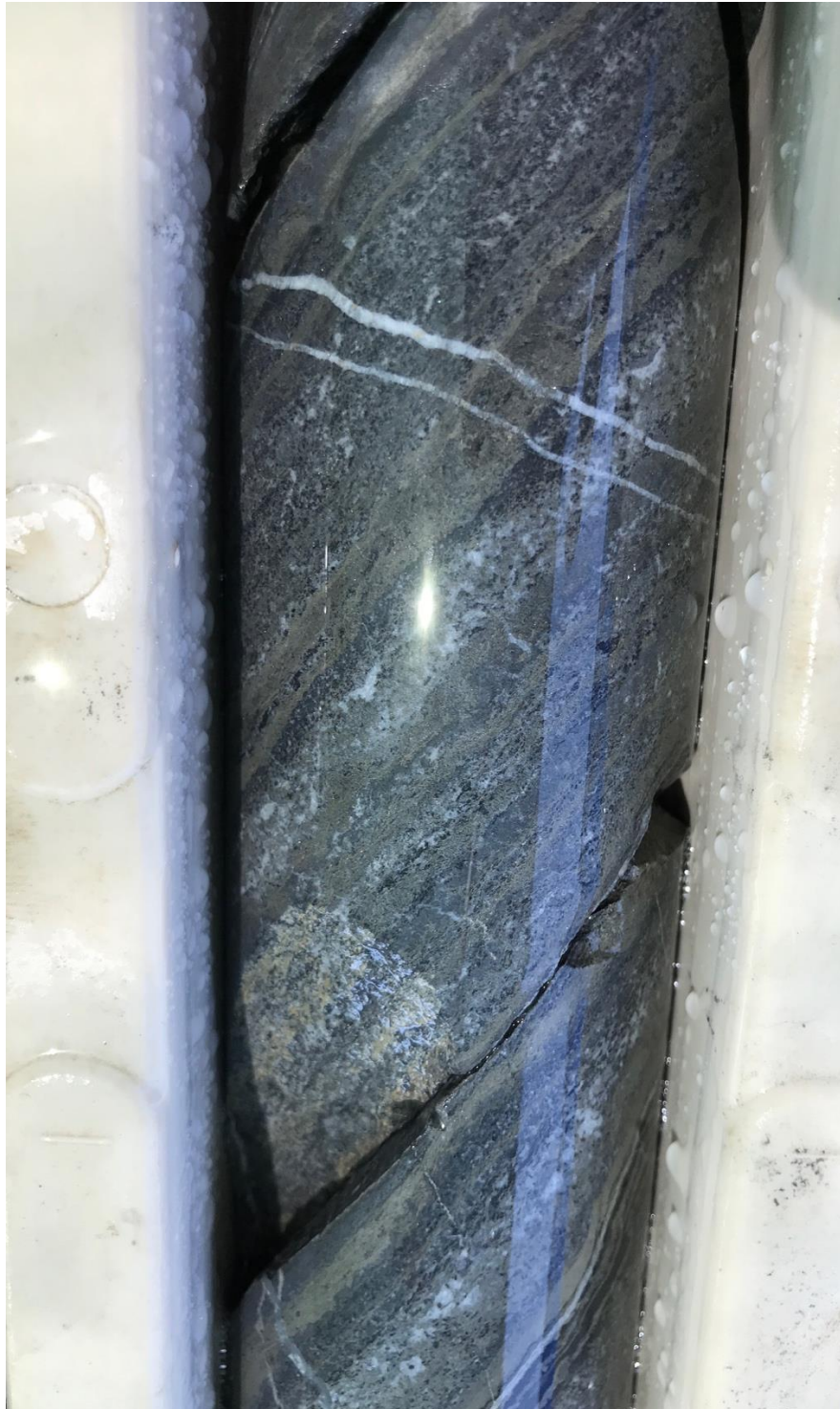
Figure Six – Fault Controlled Zinc and Lead Mineralisation in Hole BB04-17
