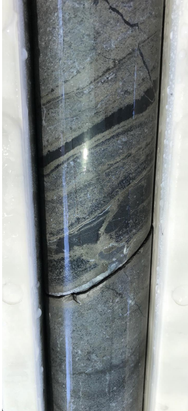
Figure Seven – Fault Controlled Zinc and Lead Mineralisation in Hole BB04-17
