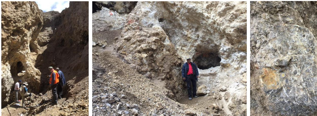
Figure 4: ABOVE LEFT One of the main excavations at Torrepatá with galleries and stopes leading from it. ABOVE MIDDLE Another excavation at Torrepatá. The pale coloring of the host limestone is due to alteration and brecciation believed associated with mineralisation. ABOVE RIGHT Detail of a mine surface that shows well developed stockwork associated with the footwall and hangingwall zones of mineralisation.
