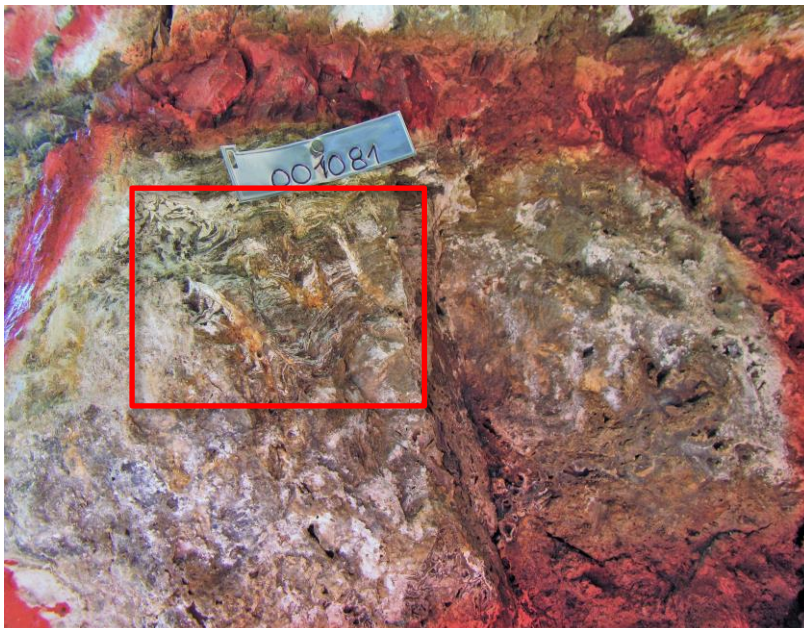
Figure 5: LEFT Sample IM-001081 (assays pending) showing smithsonite with its characteristic wavy appearance (highlighted where it is particularly concentrated) occurring at the SE most mine working, Wari.
