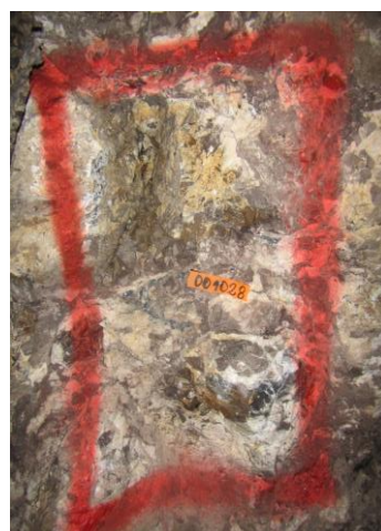
Figure 6: FAR LEFT The adit to the Torrepatá underground mine workings. A pick-up is highlighted in the background, LEFT Location of channel sample IM-001028 from gallery 1 at Torrepatá. The photo shows limestone that has intensive stockworking and dolomitic alteration over a width of 0.6m. IM-001028 contains 32.52% Pb and 18.2g/t Ag (ASX announcement 6 October 2017).
