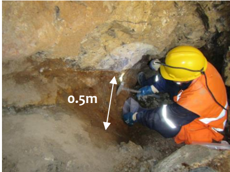
Figure 7: LEFT Preparing channel sample IM-001077 at Wari. The photo shows a 0.5m wide mineralised vein that is highly ferruginous which makes it red-brown in appearance (similar to the Vilcapuquio breccia veins). IM-001077 contains visible galena and smithsonite. ASSAYS PENDING.
