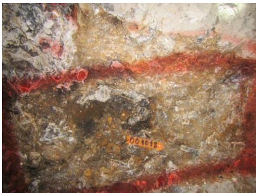
Figure 2: LEFT: Location of channel sample IM-001012, marked out in red paint, from gallery 2 at Vilcapuquio. The photo shows a breccia vein comprising clasts of limestone with a matrix of calcite, smithsonite and Fe-oxides. IM-001012 contains 33.6% Zn, 7.78% Pb and 6.4g/t Ag (ASX announcement 6 October 2017).
