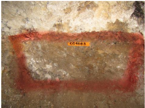
Figure 4: LEFT: Location of channel sample IM-001008 from gallery 1 at Vilcapuquio. The photo shows a breccia vein comprising clasts of limestone with a matrix of calcite with stronger Fe-oxides than IM-001002. IM-001008 contains 18.57% Zn, 19.86% Pb and 10.3g/t Ag (ASX announcement 6 October 2017).
