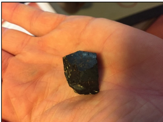
Photo 1: From PEG003, crystalline tantalum-containing mineral columbite.
