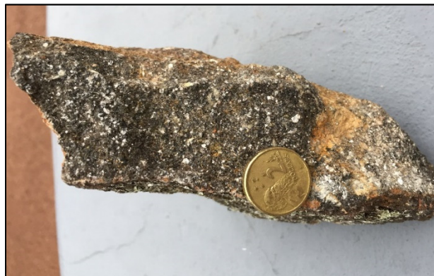
Photo 2: Micaceous LCT pegmatite from PEG003 assayed 0.72% \text{Cs}_2\text{O} , 2.91% \text{Li}_2\text{O} , and 243 ppm Ta.
