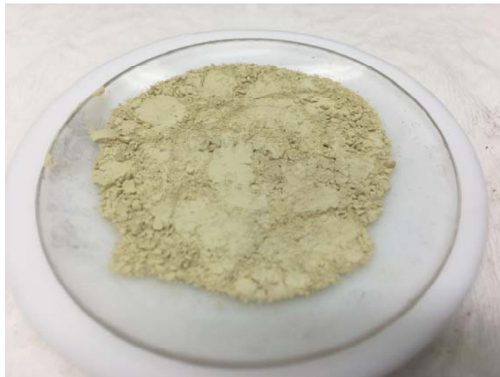
Washed Titanium Dioxide Precipitate assaying 94.5% TiO 2
