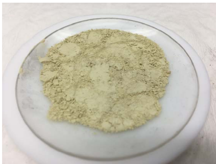
Washed Titanium Dioxide Precipitate assaying 94.5% TiO 2
